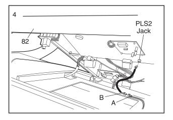
Make sure that no wires are pinched. See step 2. Reattach the Console (81) with the screws. Important: If the screws are not put back into the same holes from which they were removed, the Console will be damaged.
